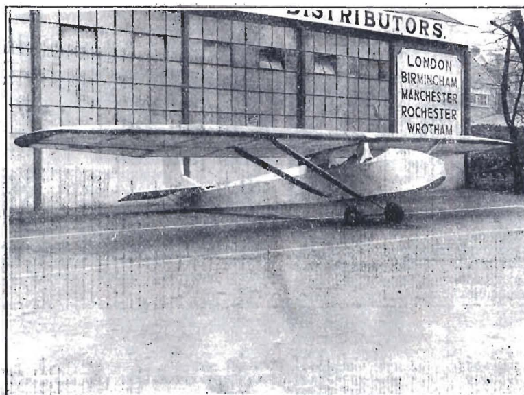
The B.A.C. VII, Two-Seat Auto-Tow Sailplane.
